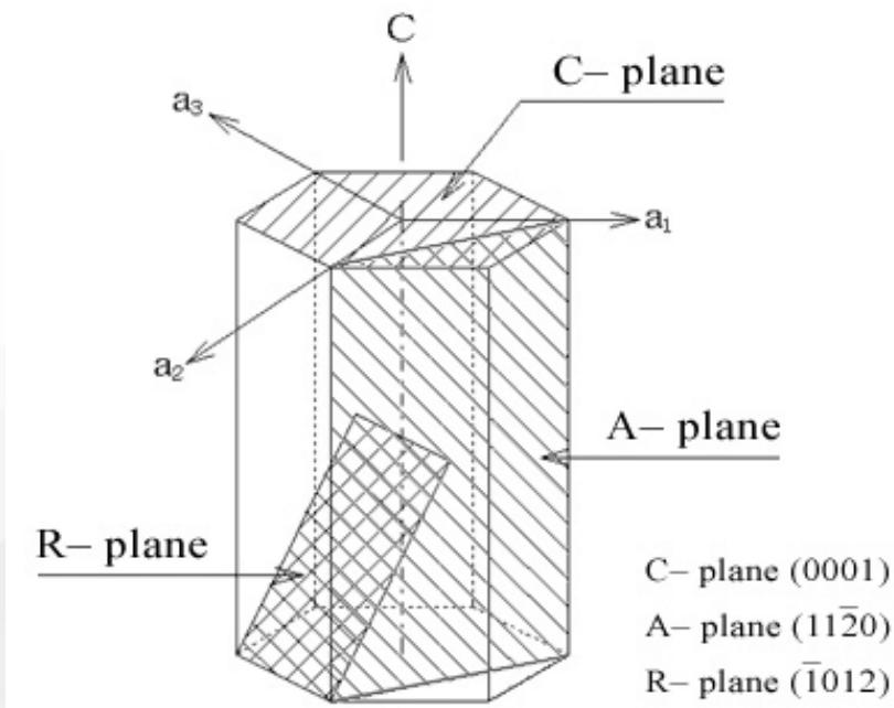
The structure of the primary planes of the sapphire crystal corresponding to the structure system of sapphire. Shown in this Figure, the C-plane is (0001), A-plane is (1120) and R-plane (1012)
